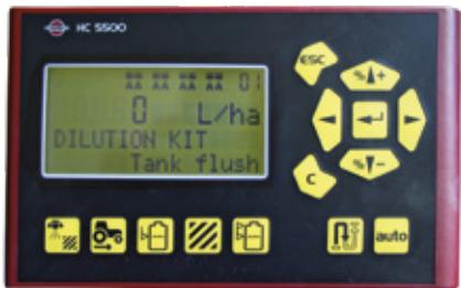
HARDI Controller for controlling spray application. The large four line display is very informative with both icons and text. It is easy add-on to the HARDI EVC control unit and can be used for GPS applications. HC 5500 can send data to a printer or a computer. The transducers based on solid state electronics.
