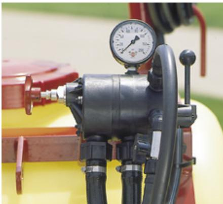
Control unit with pressure gauge made of hard wearing synthetic materials for long life and chemical resistance.
