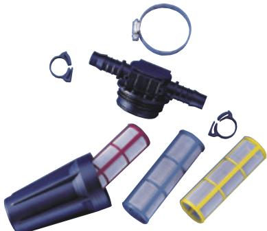
This bowl type filter is typically fitted to each boom line. It is easy to dismantle due to the radial sealing system making it quick to clean. It is available in different mesh sizes, the higher the number, the finer the mesh.
