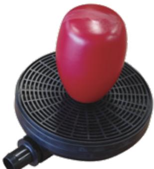
The specially designed floating suction filter aspirates water 15 cm under the surface thereby avoiding mud and surface weeds. Only clean water is sucked into the tank. Hose tail is 1½".
