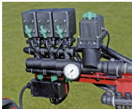
Remote controlled units utilize 12 Volt motorized valves (not solenoid) to operate the spray functions. It is the best choice for maximum operator comfort and safety.
