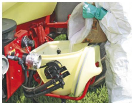
A high capacity venturi system for transferring all types of crop protection chemicals be it liquids, powders or granules to the tank. It consists of a hopper with lid, valve set and cleaning pipe.
