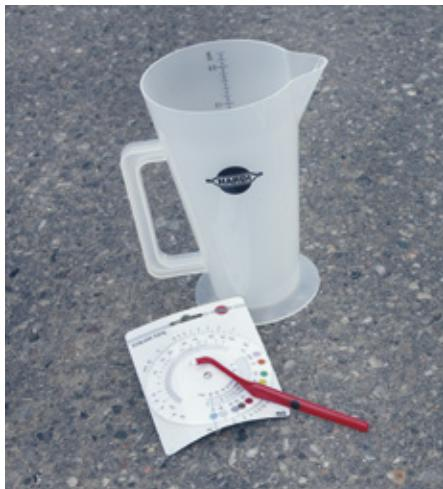
A quality kit for calibration is indispensable when using application equipment for quick and easy calculations of application rate, speed, ISO nozzle size and pressure.
